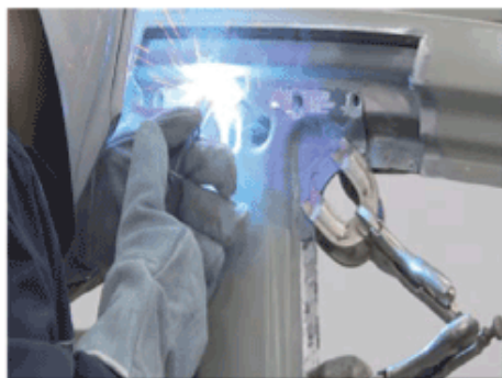
MIG Plug welding process
