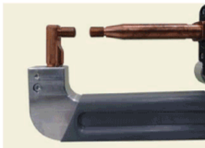
Check for contamination of welding arm (tip)
