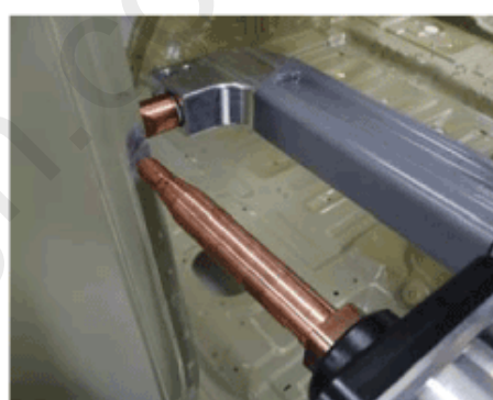
Example of panel welding (flowing current, setting)
