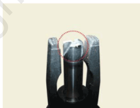
Damaged blade of carbide solid drill bit
