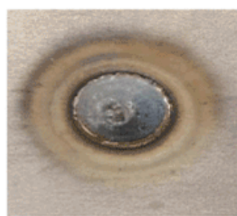
Ultra high strength (hot stamped) steel bead
