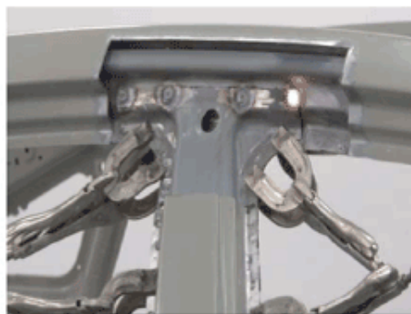
MIG Plug welding installation
