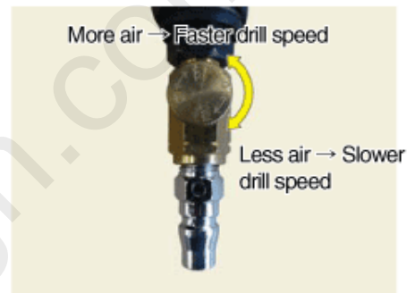
Example of installing air control valve
