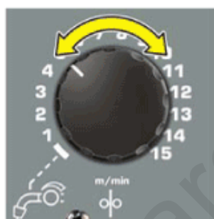
Adjust feeder speed
